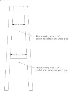
**Step 3.**Connect leg frames with 4" top braces.
